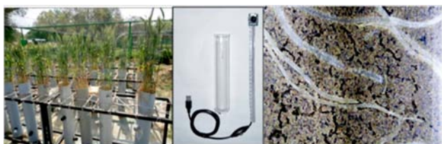
Wheat plants growing in tube rhizotron (left). The rhizotron components include - PVC pipes, glass tube and web camera (middle). A snapshot of wheat roots (right)
