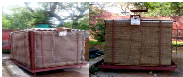
Solar powered evaporatively cooled storage structure
