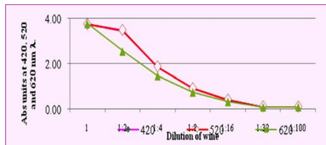
Indicative color stability: Co-pigmentation effect, in red wine from Pusa Navrang grapes after racking (69 D from start of fermentation)
