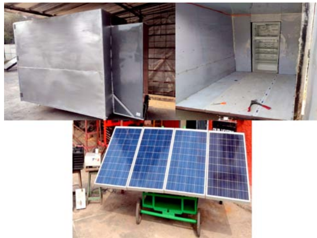
Solar powered refrigerated storage system with solar power pack
