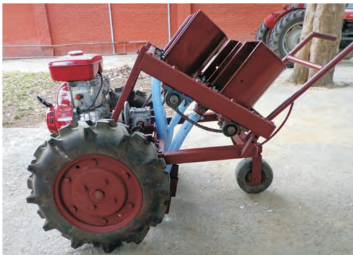
Fig. 6. Development of Self Propelled Garlic Planter
