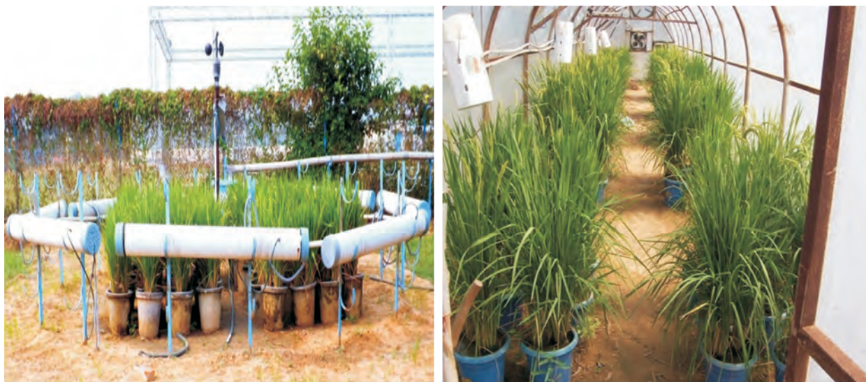
Fig. 1: Rice plants grown in elevated \text{CO}_2 (in FACE) and temperature (in TGT) conditions
