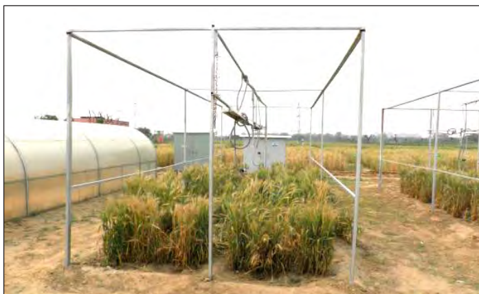
Fig. 4: Free Air Temperature Increment (FATI) facility for inducing high temperature stress on wheat crop at the experimental farm of the Agricultural Physics.
