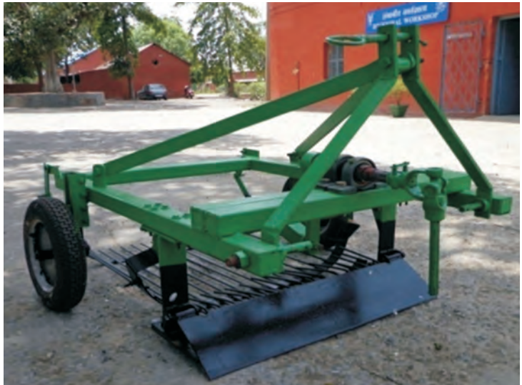
Fig. 7 Oscillating Soil Separator for Garlic Harvester
