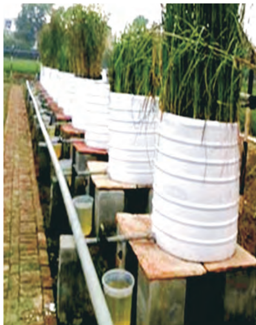
Fig. 16: Treatment cells planted with Typha latifolia , Phragmites karka , Acorus calamus
