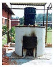
Fig. 6. Low-cost pyrolysis klin for preparation of biochar (Courtesy: T.J. Purakayastha, IARI, New Delhi)
