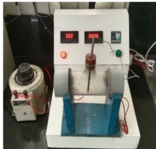
Ohmic assisted extraction technology
